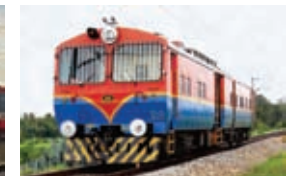
OHE Inspection Car
